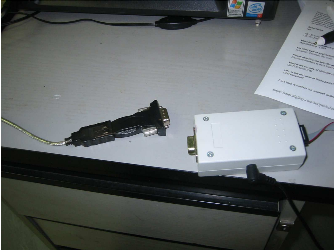
Figure 4.4.2 – Example of the serial connection removed from the SPC-1 box.
